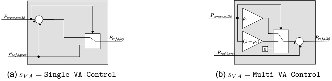
Figure 4.8: P_{ref,i} blocks for the two steady state s_{VA} states. The rest of the states are placed in appendix A.
