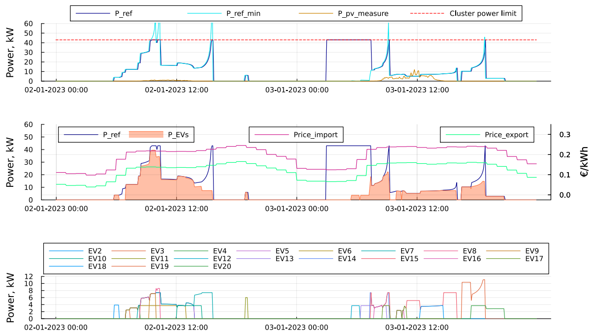
Figure 16: Winter case. Upper: Power reference allocated with P_{ref\_min} , PV measurements and cluster power limit; middle: power reference with electricity prices and aggregated power consumption of EVs; down: power consumption of each EV.
