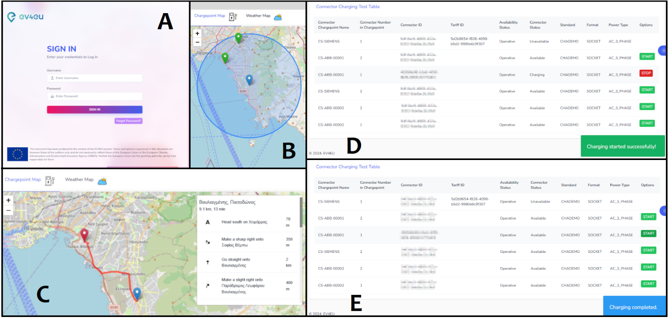
Figure 7: Summary of the main user functionalities: (A) log in, (B) search for the nearest EV chargers, (C) get directions for the selected charger, (D) start charging, after having plugged the EV, and (E) complete the charging session.
