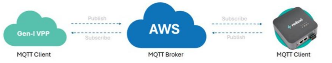
Figure 7: Concept of MQTT communication protocol
