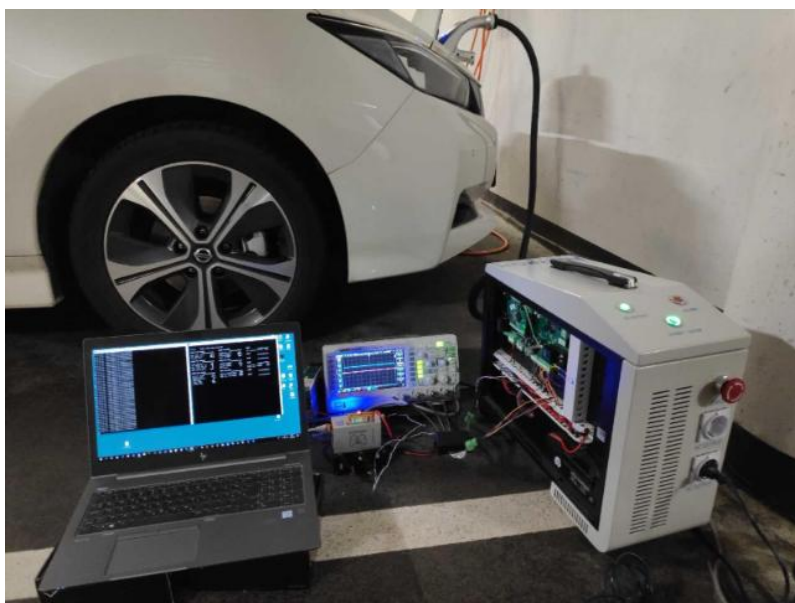
Figure 45: Testing discharging with CHAdeMO - Nisan Leaf
